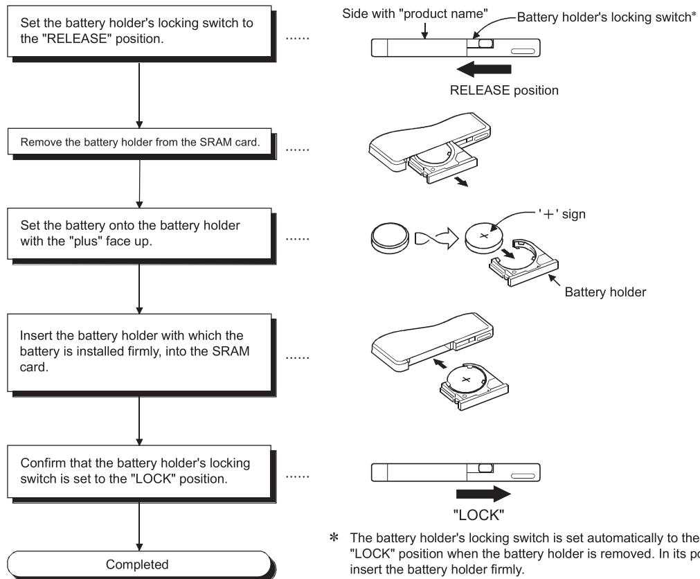
\* The battery holder's locking switch is set automatically to the "LOCK" position when the battery holder is removed. In its position, insert the battery holder firmly.
